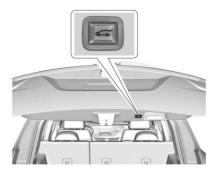
Press on the bottom of the tailgate next to the pull cup to close. Press any tailgate button, or the touch pad, or  $\mathcal{L}$  on the RKE transmitter while the tailgate is moving to stop it. Press any tailgate button again or press  $\mathcal{L}$  twice quickly on the RKE transmitter to restart the operation in the reverse direction. Pressing the touch pad on the tailgate handle will restart the motion, but only in the opening direction.
