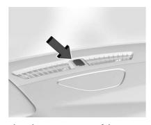
The solar sensor, on top of the instrument panel near the windscreen, monitors the solar intensity.
