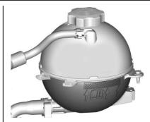
Check to see if coolant is visible in the coolant surge tank. If the coolant inside the coolant surge tank is boiling, do not do anything else until it cools down. If coolant is visible but the coolant level mark is not at or above the indicated mark, add a 50/50 mixture of clean, drinkable water and DEX-COOL coolant. Be sure the cooling system is cool before this is done. See *Engine Overheating* \$\dip 295\$.
