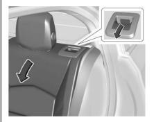
3. Pull on the lever on the top of the backrest to unlock it and fold the backrest forward
