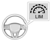
The speed limiter button is located on the steering wheel.
