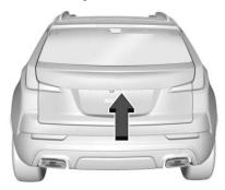
To open the tailgate, press on the power door lock switch or press on the RKE transmitter twice to unlock all doors. Press the touch pad on the underside of the tailgate handle and lift up.
