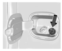
The blue AdBlue cap is behind the fuel/AdBlue hatch. If equipped with a fuel cap, do not remove the fuel and AdBlue caps at the same time. Fill diesel fuel and AdBlue independently. Turn the AdBlue cap anticlockwise to remove
