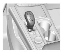
The shift pattern is displayed in the top of the gear lever. The selected gear position will illuminate red on the gear lever, while all others will be displayed in white. If the gear change is not immediate, as in very cold
