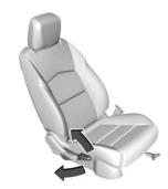
Move the lever up or down to raise or lower the seat.
