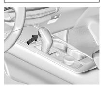
This vehicle is equipped with an electronically controlled transmission. The shift lock release button is designed to prevent inadvertent shifting out of P (Park) unless the ignition is on, the brake pedal is applied, and the shift lock release button is pressed.
