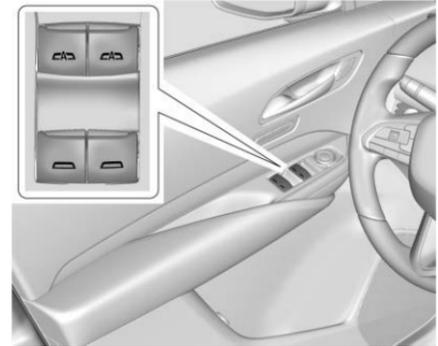
The power windows work when the ignition is on, in ACC/ACCESSORY, or when Retained Accessory Power (RAP) is active. See *Retained Accessory Power (RAP)* ⇨ 169.
