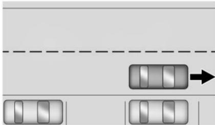
After completely passing a sufficiently large space, an audible beep occurs. A red stop symbol and a shift to reverse message are displayed.
