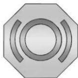
The brake master cylinder reservoir is filled with GM approved DOT 3 brake fluid as indicated on the reservoir cap. See *Engine Compartment Overview* ⇨ 246 for the location of the reservoir.
