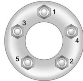
14. Tighten the wheel nuts firmly in a crisscross sequence, as shown.
