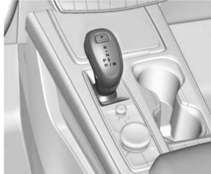
The shift pattern is displayed in the top of the gear lever. The selected gear position will illuminate red on the gear lever, while all others will be displayed in white. If the shift is not immediate, as in very cold conditions, the indicator on the gear lever may flash until it is fully engaged.
