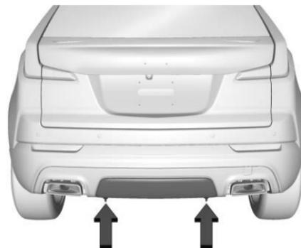
1. Remove the fasteners to remove the trailer hitch cover.
