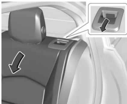
3. Pull on the lever on the top of the backrest to unlock it and fold the backrest forward.
