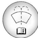
Open the cap with the washer symbol on it. Add washer fluid until the tank is full. See *Engine Compartment Overview* ⇨ 246 for reservoir location.
