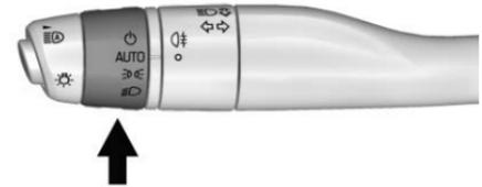
The exterior lamp control is on the indicator lever.
