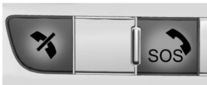
The eCall system can also be activated manually. Press
