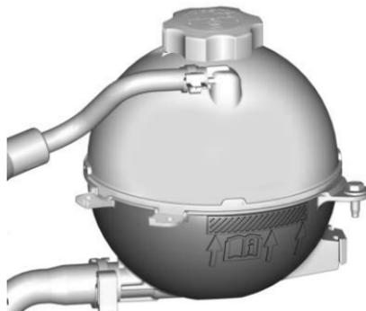
Check to see if coolant is visible in the coolant surge tank. If the coolant inside the coolant surge tank is boiling, do not do anything else until it cools down. If coolant is visible but the coolant level mark is not at or above the indicated mark, add a 50/50 mixture of clean, drinkable water and DEX-COOL coolant. Be sure the cooling system is cool before this is done. See *Engine Overheating* ⇨ 255.
