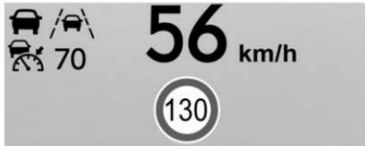
**Speed View :** This displays digital speed in English or metric units, speed limit, and indicators such as vehicle ahead, Lane Departure Warning/Lane Keep Assist, and Adaptive Cruise Control and set speed. Some information only appears on vehicles that have these features, and when they are active.
