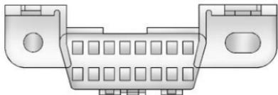
The DLC is under the instrument panel to the left of the steering wheel. Connecting devices that are not used to perform an Emissions Inspection/Maintenance test or to service the vehicle may affect vehicle operation. See *Add-On Electrical Equipment* ⇨ 240. See your dealer if assistance is needed.
