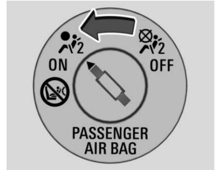
To turn the front outboard passenger airbag on again, insert the ignition key into the airbag on-off switch, push in, and move the switch to the ON position.
