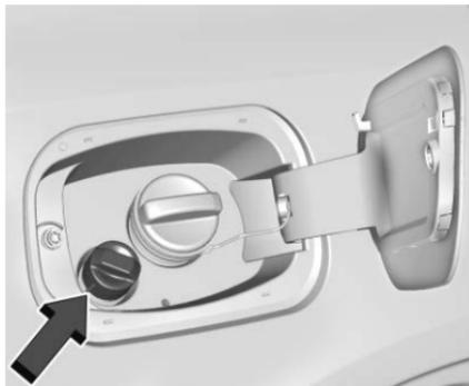
The blue DEF cap is behind the fuel/DEF door. Do not remove the fuel and DEF caps at the same time. Fill diesel fuel and DEF independently. Turn the DEF cap anticlockwise to remove.
