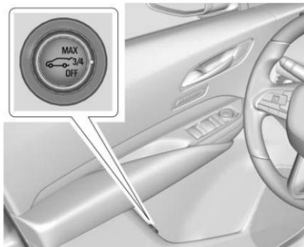
The power tailgate switch is on the driver door. The vehicle must be in P (Park).
