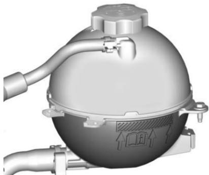
3. If topping up the level in the coolant surge tank, add the proper mixture until the level reaches the mark on the front of the tank and replace the cap. Operate the vehicle. Repeat steps 1–3, as necessary.
