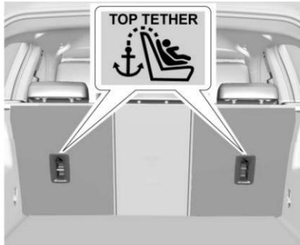
Top tether anchors are located on the back of the second row backrests and are always aligned with rear seats and identified with symbol
