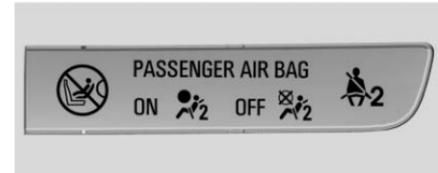
When the vehicle is started, the passenger airbag status indicator symbols for on and off will light for several seconds as a system check. Then, after several more seconds, the status indicator will light either the on or off symbol to let you know the status of the front outboard passenger frontal airbag.
