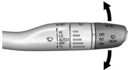
The rear window wiper/washer controls are on the end of the windscreen wiper lever.
