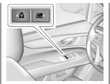
Press at to activate the safety locks on the rear doors. The indicator light comes on when activated.
