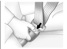
To unlatch the belt, push the button on the buckle. The belt should return to its stowed position.
