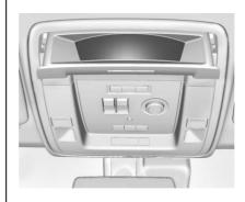
If equipped, the child-view mirror is on the overhead console. Press the fixed button on the cover to release. Push the mirror back up when not in use.
