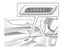
If equipped, memory seats allow two drivers to store and recall their unique seat positions for driving the vehicle, and a shared exit position for getting out of the vehicle. Other feature positions may also be set, such as power mirrors, power steering wheel, and adjustable pedals, if equipped. Memory positions are linked to RKE transmitter 1 or 2 for automatic memory recalls.
