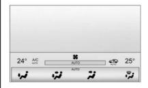
The climate control status display appears briefly when the climate control buttons on the centre console are adjusted. The air delivery mode can be adjusted on the climate control display.
