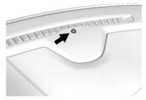
The vehicle has a light sensor on the top of the instrument panel that controls the automatic headlamp system. Do not cover the sensor, otherwise the headlamps may come on when they are not needed.
