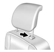
The third row seat head restraint can be lowered to allow for better visibility when the rear seat is unoccupied. To lower the head restraint, press the button located on the top of the backrest and push the head restraint down.
