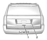
To open the tailgate, press on the power door lock switch or press on the RKE transmitter twice to unlock
