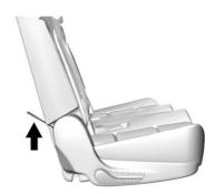
Pull the strap on the bottom rear of the second row seat to release the backrest. The seatback will fold forward.
