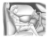
If a person of adult size is sitting in the front outboard passenger seat, but the off indicator is lit, it could be because that person is not sitting properly in the seat or that the child restraint locking feature is engaged.
