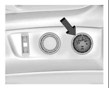
If equipped, use the transfer case knob next to the steering wheel to shift into and out of four-wheel drive.
