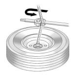
Use the wheel wrench hook to pull the hoist cable closer to assist in reaching the spare tyre.
