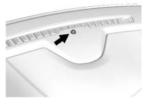
The solar sensor, on top of the instrument panel near the windscreen, monitors the solar heat.
