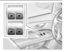
Power windows work when the ignition is on, in ACC/ACCESSORY, or when Retained Accessory Power (RAP) is active. See Retained Accessory Power  $(RAP) \Rightarrow 205$ .
