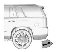
To operate, move your foot in a forward kicking motion under the centre of the rear bumper, then pull it back.
