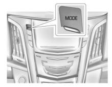
The vehicle is normally in Tour Mode. Sport Mode and Snow/Ice Mode are engaged when the Magnetic Ride Control MODE button on the centre console is pressed. Press the button to select the desired mode.
