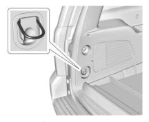
There are four cargo tie-downs in the rear cargo area. These can be used to strap cargo down and keep it from moving inside the vehicle.
