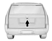
The camera that provides the Rear Camera Mirror (RCM) image is above the license plate, next to the Rear Vision Camera (RVC).
