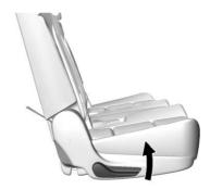
Lift the lever on the outboard side of the seat.
