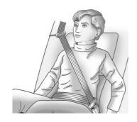
4. Buckle, position, and release the seat belt as described previously in this section. Make sure the shoulder portion of the belt is on the shoulder and not falling off of it. The belt should be close to, but not contacting, the neck. To remove and store the comfort guide, squeeze the belt edges together so that the seat belt can be removed from the guide. Slide the guide onto its storage clip.
