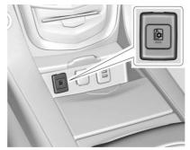
If equipped, press to turn on the cooled compartment inside the centre console storage.
