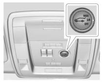
The switch is on the overhead console. The vehicle must be in P (Park).
