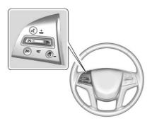
(S): Press to turn the system on and off. A white indicator appears in the instrument cluster when cruise is turned on.
