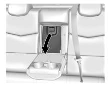
The vehicle has a rear seat pass-through door in the centre of the rear backrest. Fold down the center armrest and pull the lever all the way down to release the door.
