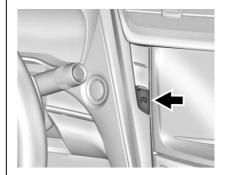
The automatic engine stop/start function can be disabled using the switch. The indicator on the switch will illuminate when the system is operational.
