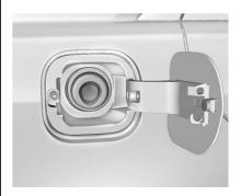
To open the fuel filler flap, push and release the rearward centre edge of the flap. The fuel door is locked when the vehicle doors are locked. Press on the RKE transmitter to unlock. See *Remote Keyless Entry (RKE) System Operation* ⇒ 28.
