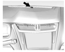
If equipped, the light sensor is on top of the instrument panel or on the windscreen near the rearview mirror.
