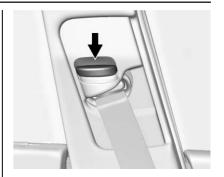
Press the release button and move the height adjuster to the desired position. The adjuster can be moved up by pushing the slide/trim up. After the adjuster is set to the desired position, try to move it down without pushing the release button to make sure it has locked into position.
