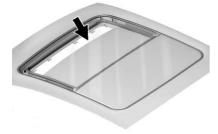
Dirt and debris may collect on the sunroof seal or in the track. This could cause an issue with sunroof operation or noise. It could also plug the water drainage system. Periodically open the sunroof and remove any obstacles or loose debris. Wipe the sunroof seal and roof sealing
