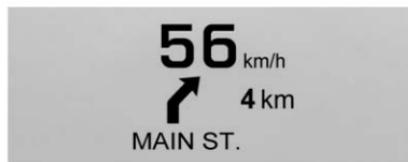
**Navigation View** : This display includes the information in the speed view along with Turn-by-Turn Navigation information in some vehicles. The compass heading is displayed when navigation routing is not active.
