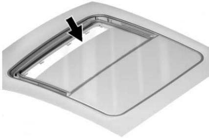
Dirt and debris may collect on the sunroof seal or in the track. This could cause an issue with sunroof operation or noise. It could also plug the water drainage system.
