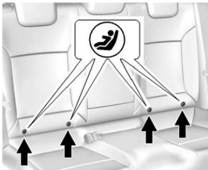
ISOFIX mounting brackets are marked by
