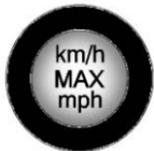
16. If the flat tyre was able to inflate to the recommended inflation pressure, remove the maximum speed label from the sealant canister (5) and place it in a highly visible location. Do not exceed the speed on this label until the damaged tyre is repaired or replaced.
