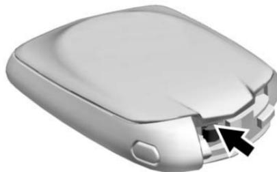
2. Separate the two halves of the transmitter using a flat tool inserted into the bottom centre of the transmitter, do not use the key slot.
