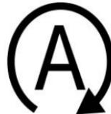
This light comes on when the engine is in an Auto Stop.
