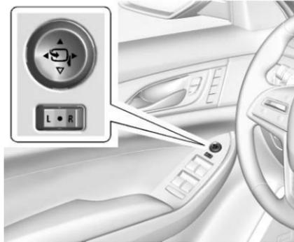
Controls for the outside power mirrors are on the driver door.
