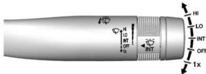
With the ignition in ACC/ACCESSORY or ON/RUN/START, move the windscreen wiper stalk to select the wiper speed.
