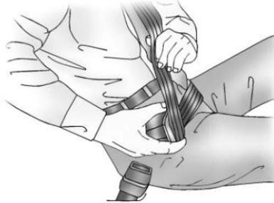
If the webbing locks in the catch plate before it reaches the buckle, tilt the catch plate flat to unlock.
