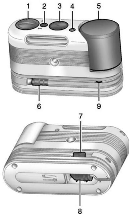
When using the tyre sealant and compressor kit during cold temperatures, warm the kit in a heated environment for five minutes. This will help to inflate the tyre faster.
