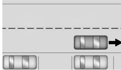
After completely passing a large enough space bordered by two vehicles or other objects, an audible beep occurs and a red symbol displays in the DIC.
