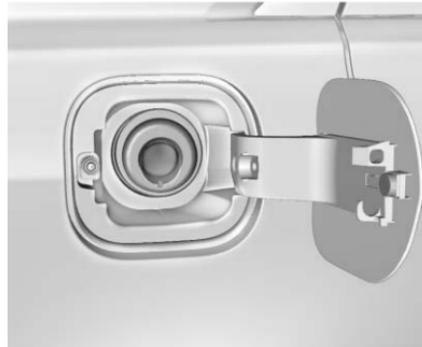
To open the fuel filler flap, push and release the rearward centre edge of the flap. The fuel door is locked when the vehicle doors are locked. Press
