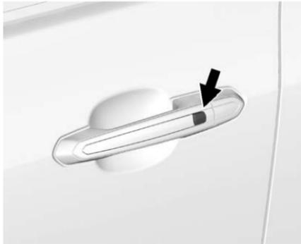
Use the Keyless Access system to lock and unlock the door. When the doors are locked and the Remote Keyless Entry (RKE) transmitter is within 1 m (3 ft) of the driver door handle, press the lock/unlock button. When unlocking from the driver door, the first press unlocks that door; press
