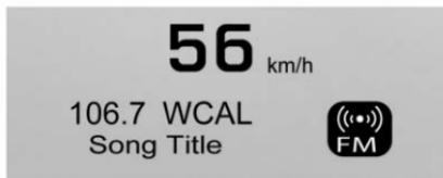
**Audio/Phone View** : This displays the speed view along with audio/phone information. The current radio station, media type, and incoming calls will be displayed when active on vehicles equipped with these features.
