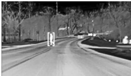
With the Front Pedestrian Braking system turned on, Night Vision provides a red Head-Up Display (HUD) alert when the system detects that the vehicle is approaching a pedestrian ahead much too quickly. In addition, an alert beeps or the Safety Alert Seat pulses, if equipped. See *Front Pedestrian Braking (FPB) System* ⇨ 232.
