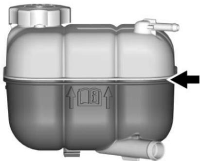
Check to see if coolant is visible in the coolant surge tank. If the coolant inside the coolant surge tank is boiling, do not do anything else until it cools down. If coolant is visible but the coolant level mark is not visible, add a 50/50 mixture of clean, drinkable water and DEX-COOL coolant at the coolant surge tank to
