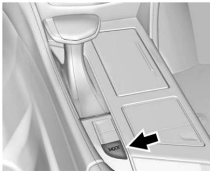
Press and release MODE on the centre console to activate the mode menu in the instrument cluster. The first press
