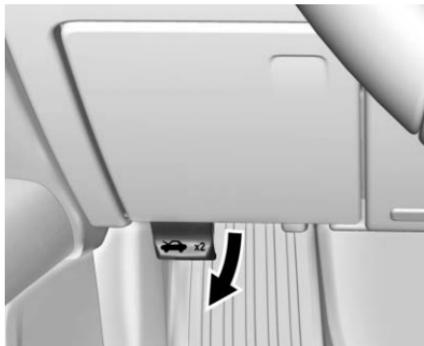
1. Pull the bonnet release handle. It is on the lower left side of the instrument panel between the door and the steering wheel.
