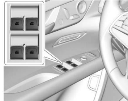
The windows work when the vehicle is in ON/RUN, ACC/ACCESSORY, or Retained Accessory Power (RAP). See *Retained Accessory Power (RAP)* ⇨ 198.
