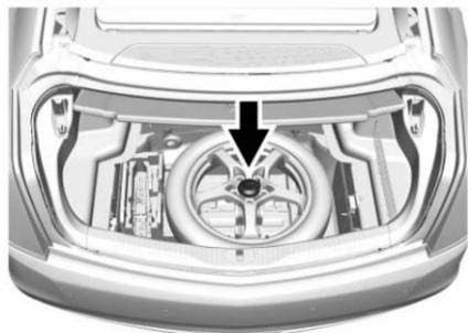
3. Turn the retainer nut anticlockwise and remove the spare tyre. Place the spare tyre next to the tyre being changed.
