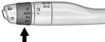
The exterior lamp control is on the indicator lever.
