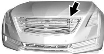
The vehicle may have a shutter system designed to help increase fuel economy. Keep the shutter system clean for proper operation.
