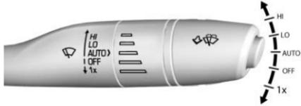
With the ignition in ACC/ACCESSORY or ON/RUN, move the windscreen wiper lever up or down to select the wiper speed.
