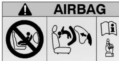
When securing a child restraint in a rear seating position, study the instructions that came with your child restraint to make sure it is compatible with this vehicle.
