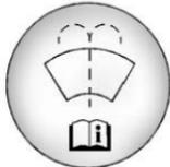
Open the cap with the washer symbol on it. Add washer fluid until the tank is full. See *Engine Compartment Overview* ⇨ 247 for reservoir location.
