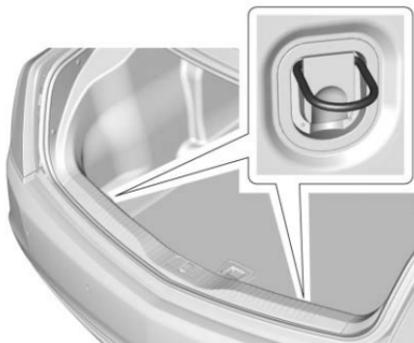
The cargo tie-downs can be used to secure small loads and the convenience net. See *Convenience Net* ⇨ 104, if equipped.
