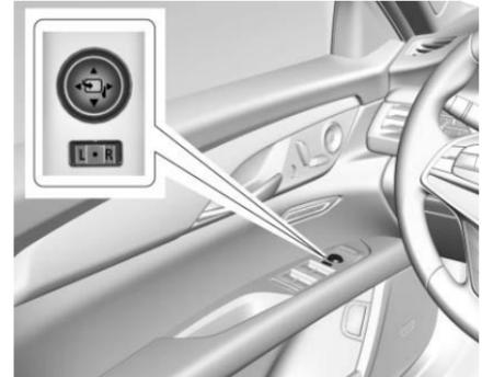
1. Move the selector switch to L (Left) or R (Right) to choose the driver or passenger mirror.
