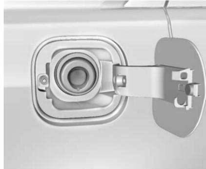
To open the fuel filler flap, push and release the rearward centre edge of the flap. The fuel door is locked when the vehicle doors are locked. Press
