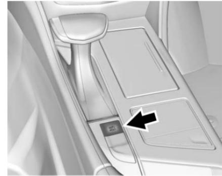
Automatic Vehicle Hold (AVH) can be turned on by pressing AUTO HOLD with the driver seat belt fastened, the driver door closed, and the engine running. The AVH indicator will come on.
