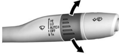
**AUTO** : Use this setting for intermittent wipes when Rainsense™ is disabled, or for Rainsense wipes when it is enabled. For intermittent wipes, move the lever up to AUTO, then turn the band on the wiper lever up for more frequent wipes or down for less frequent wipes. If Rainsense is enabled, see “Rainsense™” later in this section.
