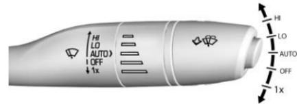
With the ignition in ACC/ACCESSORY or ON/RUN, move the lever up or down to select the wiper speed.
