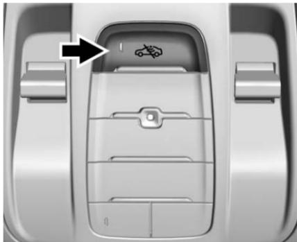
With the vehicle turned off, press
