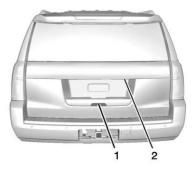
To open the tailgate, press on the power door lock switch or press on the RKE transmitter twice to unlock all doors. Press the touch pad (1) on the underside of the tailgate handle and lift up.
