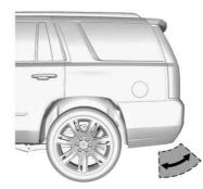
To operate, move your foot in a forward kicking motion under the centre of the rear bumper, then pull it back.
