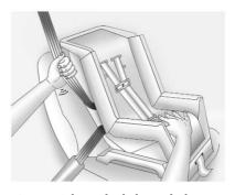
. To tighten the belt, push down on the child restraint, pull the shoulder portion of the belt to tighten the lap portion of the belt, and feed the shoulder belt back into the retractor. When installing a forward-facing child restraint, it may be helpful to use your knee to push down on the child restraint as you tighten the belt.
