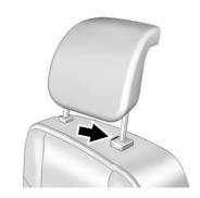
The third row seat head restraint can be lowered to allow for better visibility when the rear seat is unoccupied. To lower the head restraint, press the button located on the top of the backrest and push the head restraint down.
