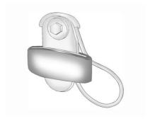
Remove the guide from its storage clip on the interior trim next to the outboard backrest.
