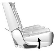
Lift the lever on the outboard side of the seat to release the seatback.
