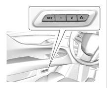
The SET, 1, 2, and (Exit) buttons on the driver's door are used to manually store and recall memory settings for the driver seat, exterior mirrors, power tilt and telescoping steering column, adjustable pedals (if equipped), and massage settings (if equipped).
