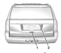
To open the tailgate, press on the power door lock switch or press on the Remote Keyless Entry (RKE) transmitter twice to unlock all doors. Press the touch pad (1) on the underside of the tailgate handle and lift up. See *Remote Keyless Entry (RKE)* System Operation ⇒ 28.
