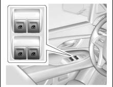
The windows work when the vehicle is in ON/RUN, ACC/ACCESSORY, or when Retained Accessory Power (RAP) is active. See *Retained Accessory Power (RAP) ⇒* 210.
