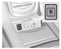
If equipped, press to turn on the cooled compartment inside the centre console storage.
