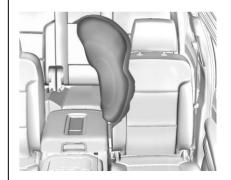
The front centre airbag is in the inboard side of the driver backrest.
