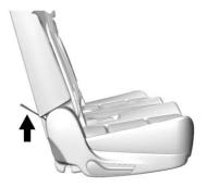
2. Pull the strap on the bottom rear of the second row seat to release the backrest. The seatback will fold forward.
