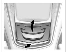
Touch the bottom of the climate control system panel until the door automatically starts to open. The storage area may contain a USB port. See the infotainment manual.
