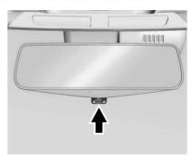
Pull the tab rearward to turn on the display. Push the tab forward to turn it off. When off, the mirror is automatic dimming. Adjust the mirror for a clear view of the area behind the vehicle while the display is off.
