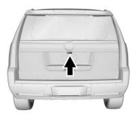
The camera that provides the Rear Camera Mirror (RCM) image is above the license plate, next to the Rear Vision Camera (RVC).
