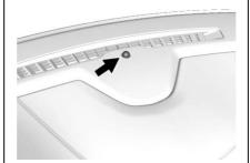
The vehicle has a light sensor on the top of the instrument panel that controls the automatic headlamp system. Do not cover the sensor, otherwise the headlamps may come on when they are not needed.
