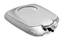
Separate the two halves of the transmitter using a flat tool inserted into the bottom centre of the transmitter. Do not use the key slot.
