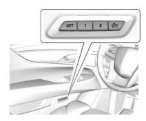
The SET, 1, 2, and (Exit) buttons on the driver door are used to manually store and recall memory settings for the driver seat, outside mirrors, power tilt and telescoping steering column, adjustable pedals (if equipped), and massage settings (if equipped).
