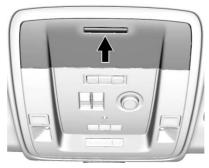
If equipped, sunglasses storage is on the overhead console. Press the fixed button on the cover and release to access. There may be a child-view mirror located within the sunglasses bin. Release the bin and then push up halfway to secure in position.
