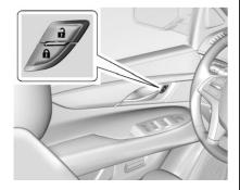
(Lock): Press to lock the doors. (Unlock): Press to unlock the doors.
