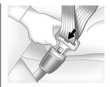
Push the latch plate into the buckle until it clicks. If you find that the latch plate will not go fully into the buckle, see if you are using the correct buckle.
