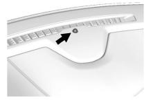
The solar sensor, on top of the instrument panel near the windscreen, monitors the solar heat.
