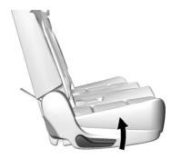
Lift the lever on the outboard side of the seat to release the seatback.
