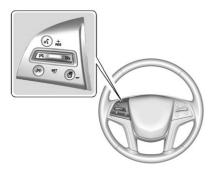
(S): Press to turn the system on and off. A white indicator appears in the instrument cluster when cruise is turned on. +RES: If there is a set speed in memory, press the control up briefly to resume that speed or press and hold to accelerate. If the cruise control is already active, use to increase vehicle speed.
