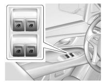
The driver's door switches control all windows. Each passenger door has a switch that controls only that window. The power windows work when the ignition is in ON/RUN or ACC/ACCESSORY, or in Retained Accessory Power (RAP). See Retained Accessory Power (RAP) ⇒ 206.
