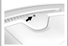
The vehicle has a light sensor on the top of the instrument panel that controls the automatic headlamp system. Do not cover the sensor, otherwise the headlamps may come on when they are not needed.
