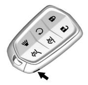
The transmitter has a button on the side used to remove the key. Do not pull the key out without pressing the button.
