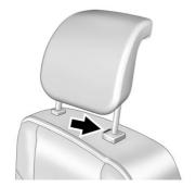
The third row seat head restraint can be lowered to allow for better visibility when the rear seat is unoccupied.
