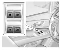
The power windows work when the ignition is in ON/RUN or ACC/ ACCESSORY, or in Retained Accessory Power (RAP). Press the switch to lower the window. Pull the switch to raise it. See Retained Accessory Power (RAP) ⇒ 206.
