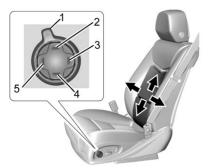
Press and release or hold Feature Select (1) to scroll to lumbar support on the centre console.
