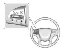
(S) (On/Off): Press to turn the system on or off. The indicator turns white on the instrument cluster when ACC is turned on.
