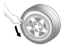
Use the wheel wrench to loosen all the wheel nuts. Turn the wheel wrench anticlockwise to loosen the wheel nuts. Do not remove the wheel nuts yet.
