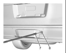
Insert the open end of the extension (7) through the hole in the rear bumper (8) (hoist shaft access hole).
