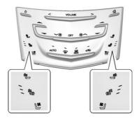
The buttons are near the climate controls on the centre stack. To operate, the engine must be running.
