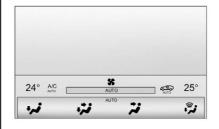
The climate control status screen appears briefly when the climate control buttons on the faceplate are adjusted. The air delivery mode can be adjusted on the climate control status screen.
