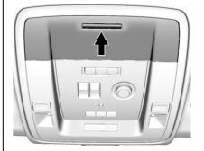
If equipped, sunglasses storage is on the overhead console. Press the fixed button on the cover and release to access. There may be a child-view mirror located within the sunglasses bin. Release the bin and then push up halfway to secure in position.
