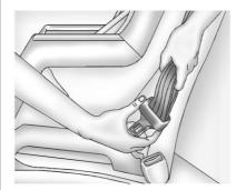
2. Pick up the latch plate, and run the lap and shoulder portions of the vehicle's safety belt
