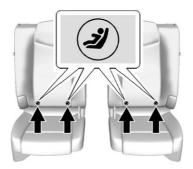
Second Row - Bucket Fasten vehicle-approved ISOFIX child restraint systems to the ISOFIX mounting brackets.
