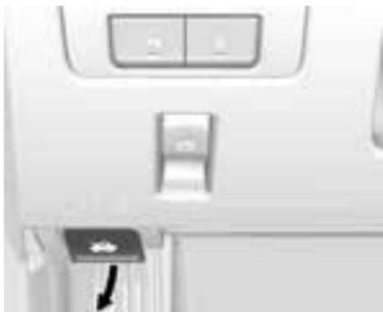
1. Pull the bonnet release handle inside the vehicle. It is on the lower left side of the instrument panel.
