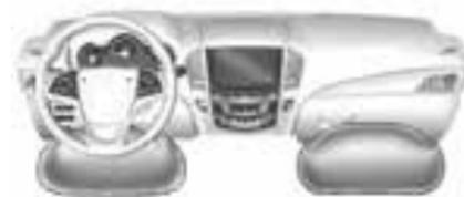
The driver knee airbag is below the steering column. The front outboard passenger knee airbag is below the glove box.
