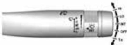
With the ignition in ACC/ACCESSORY or ON/RUN/START, move the stalk to select the wiper speed.
