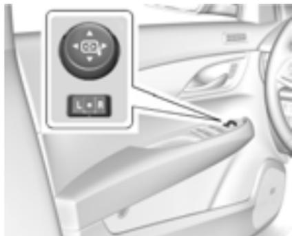
1. Move the selector switch to L (Left) or R (Right) to choose the driver or passenger mirror.
