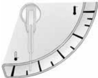
This gauge measures the temperature of the vehicle's engine. If the needle moves into the shaded area while driving under normal operating conditions, the engine is
