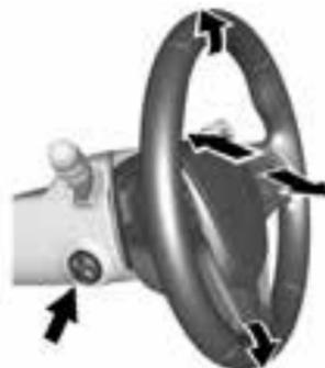
If equipped, the control is on the left side of the steering column.
