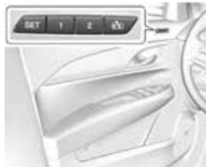
If equipped, the "1," "2," SET, and
