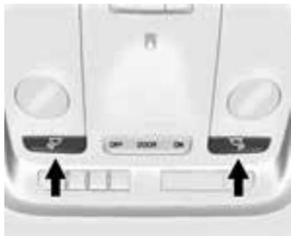
The front reading lamps are in the overhead console.
