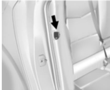
1. Remove the guide from its storage pocket on the side of the seat.
