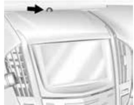
The solar sensor monitors the solar heat.
