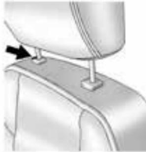
To lower the outboard head restraint, press the button, located on the top of the seatback, and push the head restraint down. Try to move the head restraint after the button is released to make sure that it is locked in place.
