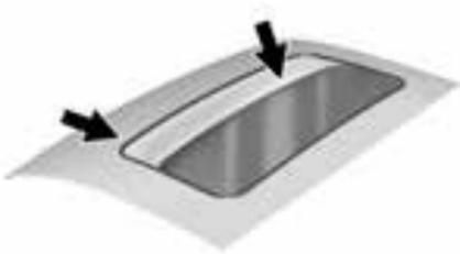
Dirt and debris may collect on the sunroof seal or in the track. This could cause an issue with sunroof operation or noise. It could also plug the water drainage system.
