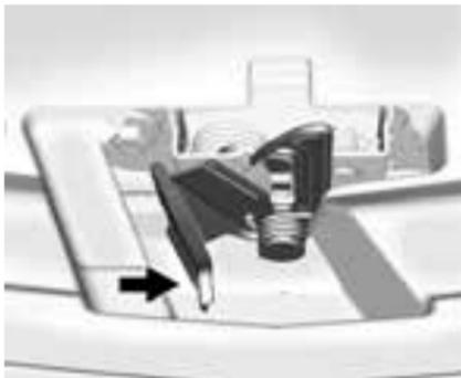
2. Go to the front of the vehicle and move the secondary bonnet release lever toward the right side of the vehicle.
