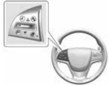
**(On/Off):** Press to turn the system on or off. A white cruise control indicator comes on.
