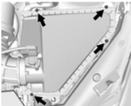
1. Remove the four screws and lift the cover out of the assembly.
