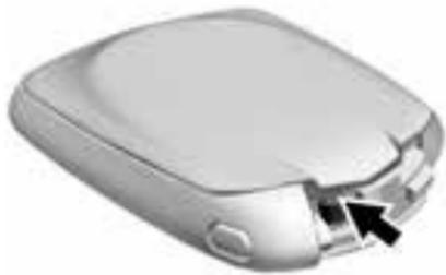
2. Separate the two halves of the transmitter using a flat tool inserted into the bottom centre of the transmitter. Do not use the key slot.
