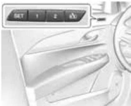
If equipped, the "1," "2," SET, and
