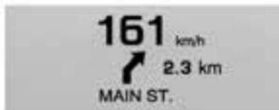
**Navigation View:** This display includes the information in speed view along with Turn-by-Turn Navigation information. The compass heading is displayed when navigation routing is not active.
