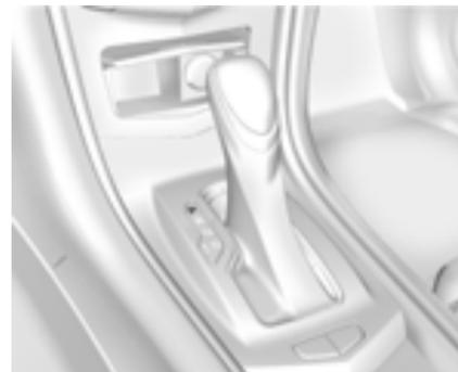
**P (Park):** This position locks the rear wheels. Use this position when starting the engine because the vehicle cannot move easily.
