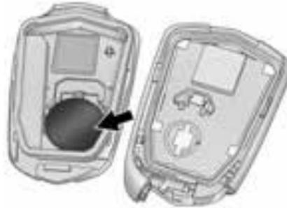
3. Remove the old battery. Do not use a metal object.
