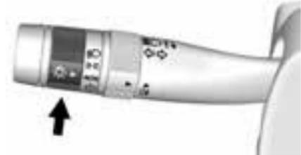
The exterior lamp control is on the indicator lever.
