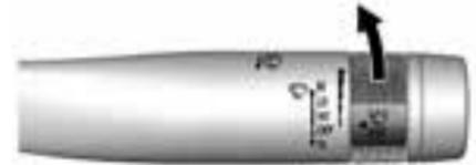
**INT (Intermittent Wiper):** Move the lever up to INT for intermittent wiper, then turn the
