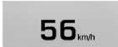
**Speed View:** This display gives the speedometer reading (in English or metric units), traffic sign memory, Adaptive Cruise Control speed, Forward Collision Alert status, Lane Departure Warning, and Vehicle Ahead indicator. Some information only appears on vehicles that have these features, and when they are active.
