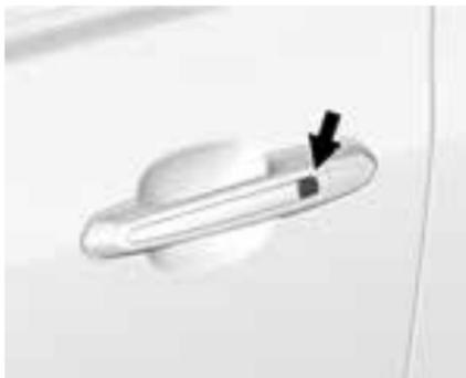
If equipped, use the Keyless Access system to lock and unlock the door. When the doors are locked and the RKE transmitter is within 1 m (3 ft) of the driver door handle, press the lock/unlock button. When unlocking from the driver door, the first press unlocks that door; press again within five seconds to unlock all passenger doors. See *Remote Keyless Entry (RKE) System Operation* on page 2-2.
